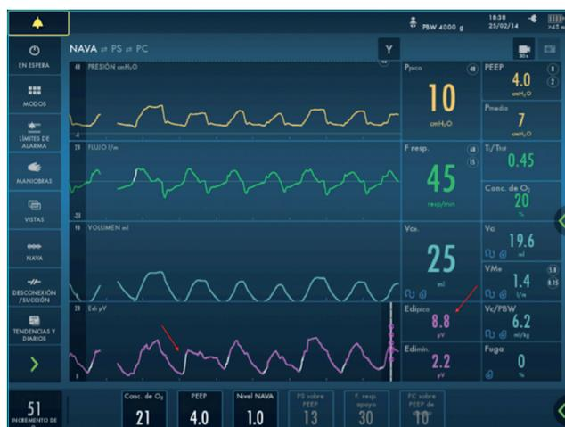
**Figure 2** Ventilation SERVO-i with NAVA display showing Edi signal (arrows).
